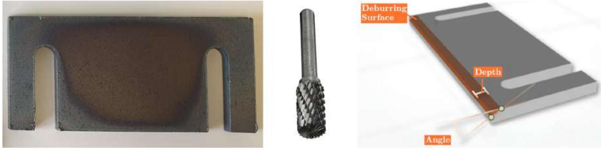
Figure 2.8: Metal workpiece considered for the deburring application (left), cylindrical drill bit (center), and determination of the deburring surface from process parameters (right).
