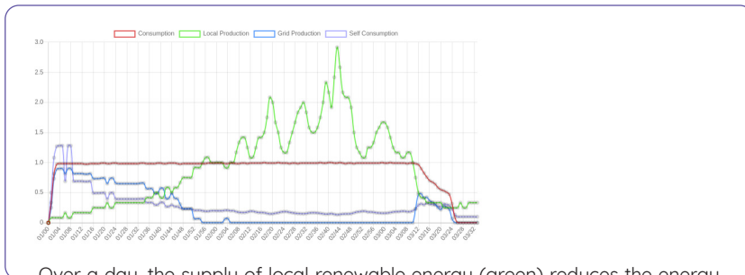
Over a day, the supply of local renewable energy (green) reduces the energy supply required from the grid (mid-blue). This can be stored for later use (e.g. overnight charging).
